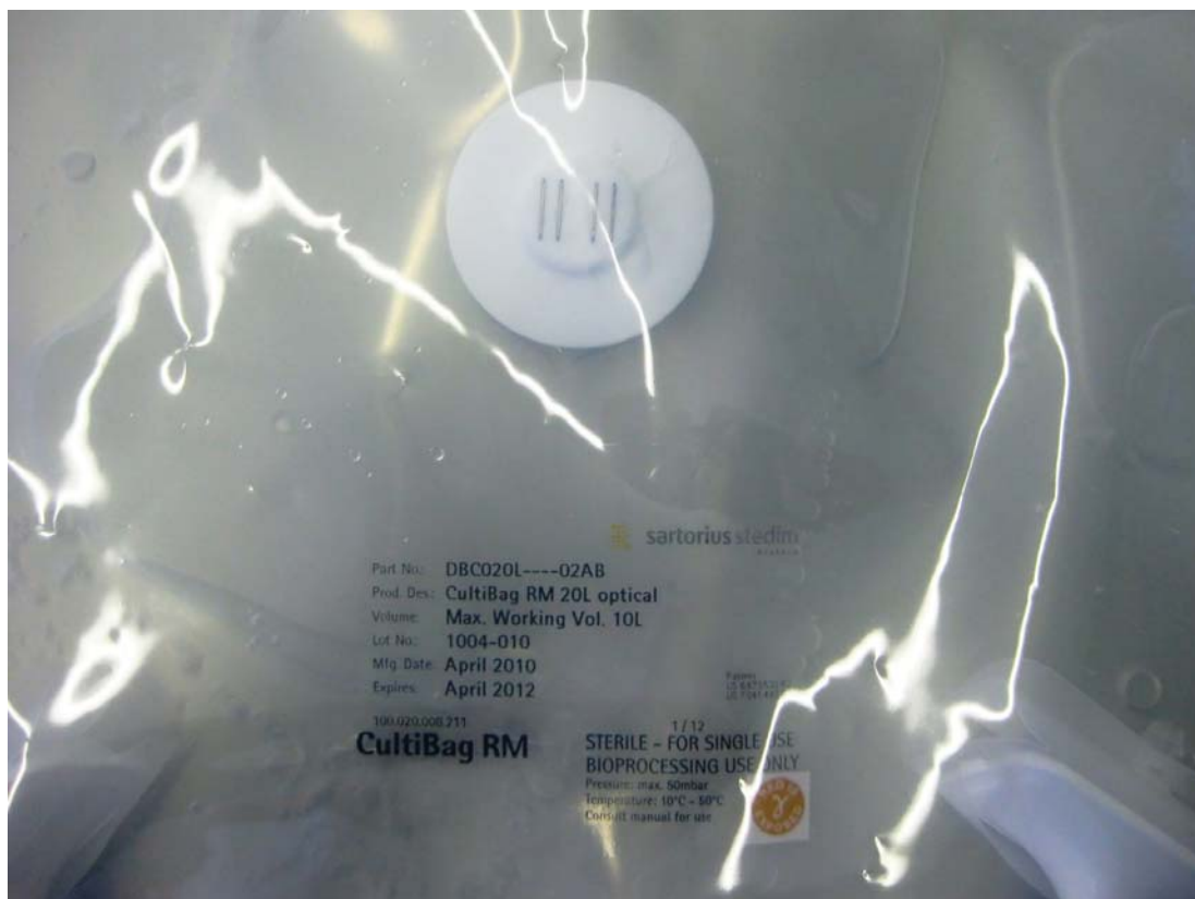
Figure 7 Aber Disposable Probe welded into a Sartorius Stedim Biotech CultiBag RM 20L optical (10 L working volume)
